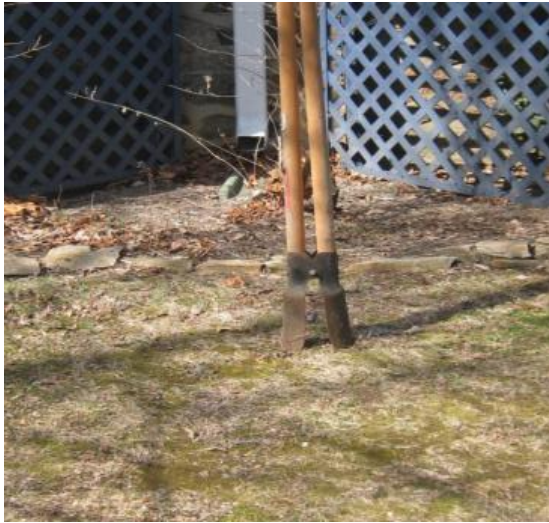
Post Hole Digger for Soil Test
