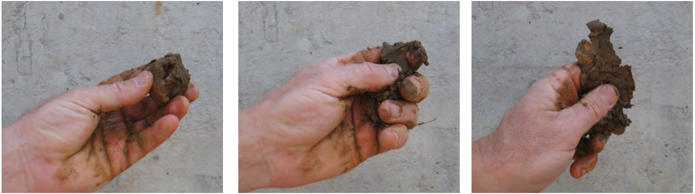
Figure B.1. Shown from left to right: Ball test, feel test, and ribbon test
